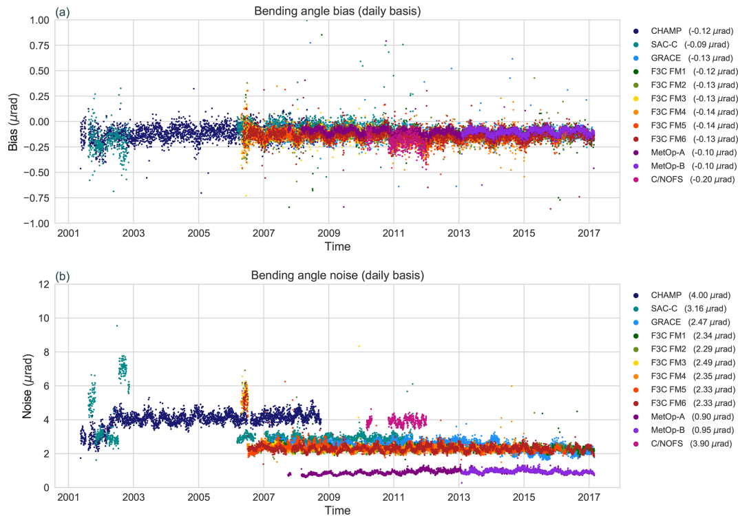
Figure 6. Temporal evolution of daily median bending angle bias (a) and bending angle noise standard deviation (b) for all RO missions used in OPSv5.6. Total mean of bending angle bias and noise is shown as a value in parentheses in the respective legend. Only high-quality profiles are used in these statistics.
