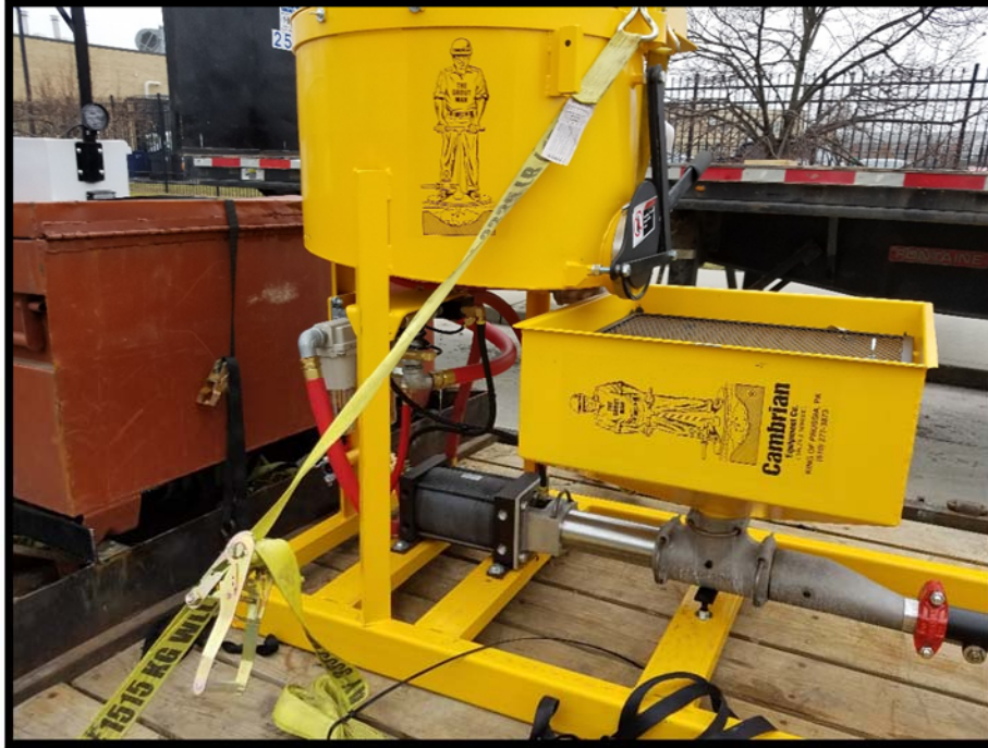
Grout mixing and pressure injection machine.
