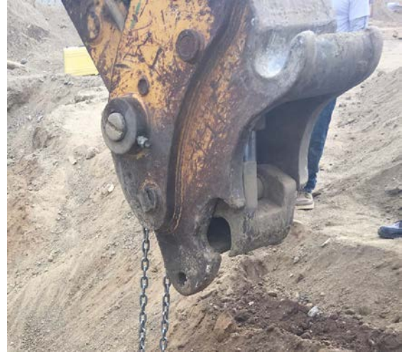
Exhibit 6. The quick coupler attached to the end of the boom.
