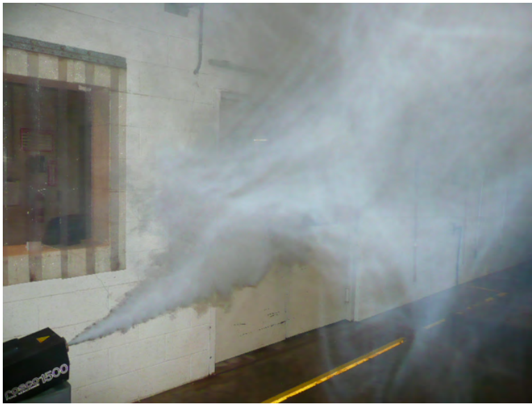
Figure 2. Theatrical smoke generated outside of the food preparation area in the phase 2 quarantine barn. Photo by NIOSH.
