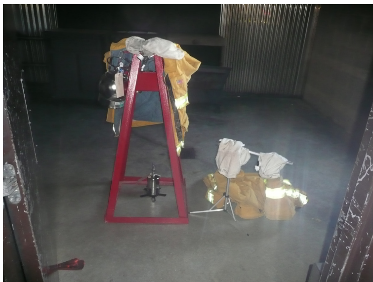
Figure 5. Area air sampling set-up for Exercise 5.
