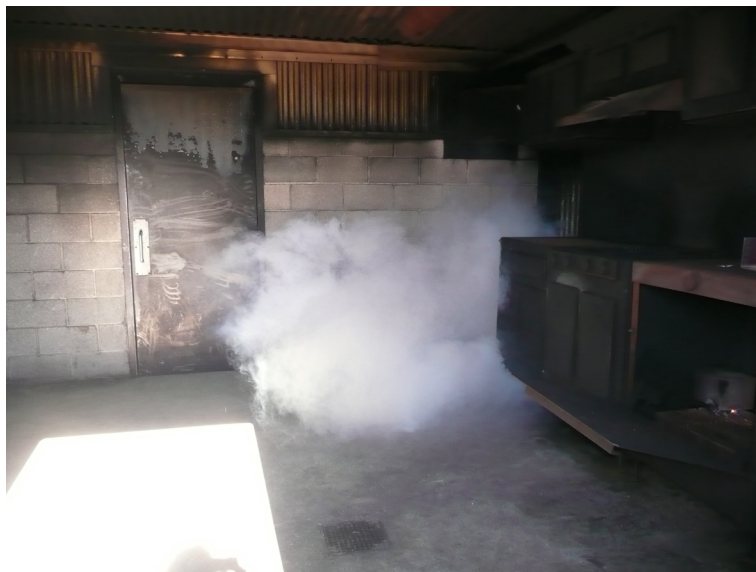
Figure 3. Mineral oil-based smoke simulant exiting the supply nozzle in the corner of the first floor training room.
