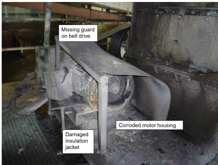
Figure 8. Corroded metal housing surrounding the shredder motor, damaged electrical insulation, and an unguarded drive belt. Photo by NIOSH.
