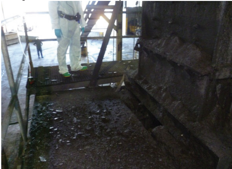
Figure 8. Corroded metal housing surrounding the shredder motor, damaged electrical insulation, and an unguarded drive belt. Photo by NIOSH.
