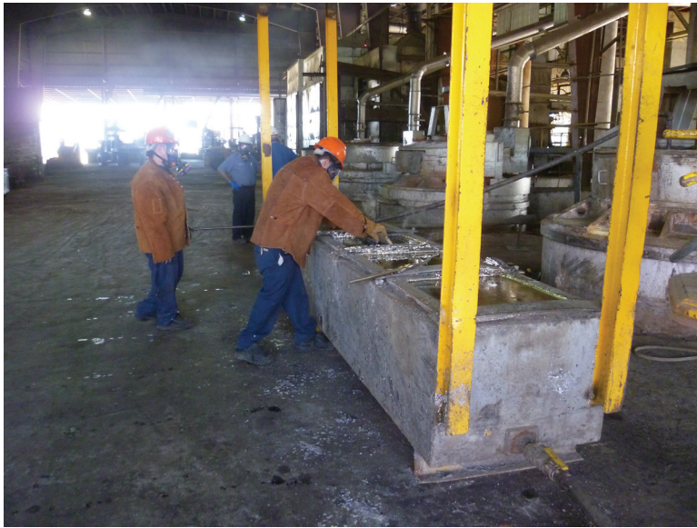
Figure 5. Employee scraping floating impurities (dross) from molten lead nuggets. Photo by NIOSH.
