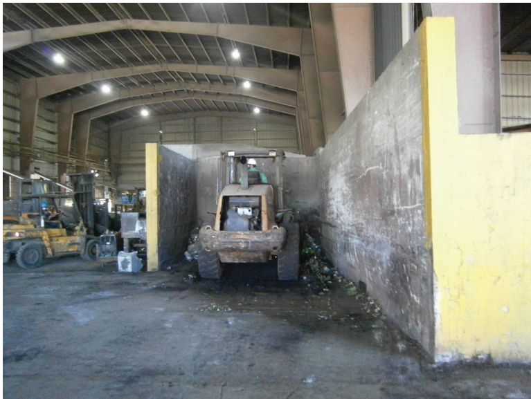
Figure 2. Area where lead-containing materials were air dried and then mixed with coal, soda ash, and scrap metal by employees using front-end loaders. Photo by NIOSH.
