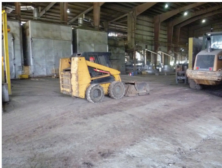
Figure 7. Employee using skid loader with rotary brush attachment to sweep dry floor. Photo by NIOSH.
