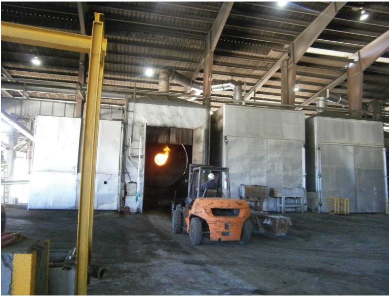
Figure 3. A front loader moving a mixture of lead-containing materials and soda ash into a furnace. Photo by NIOSH.
