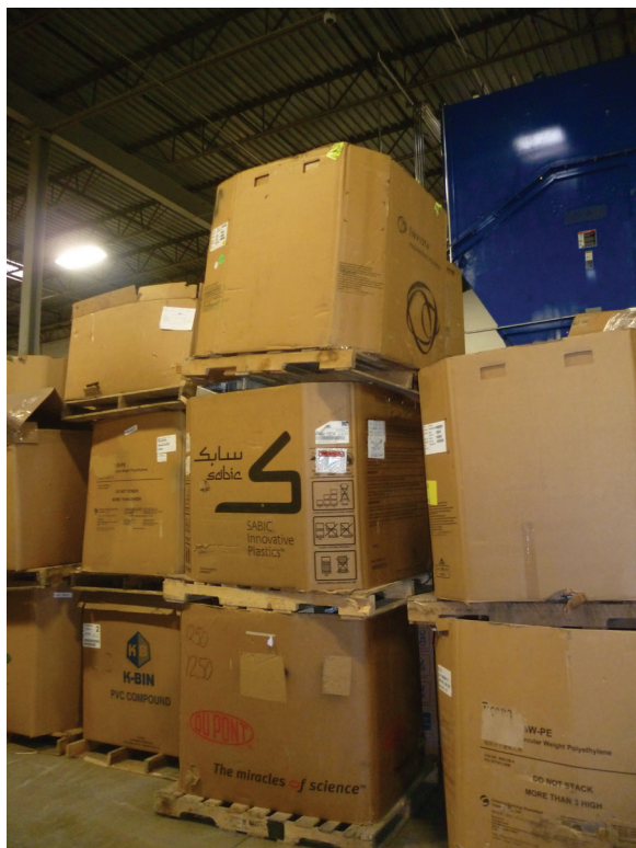
Figure 10. Large poorly stacked cardboard boxes filled with electronic scrap. Photo by NIOSH.
