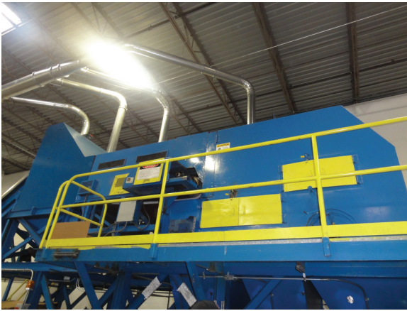
Figure 6. Eddy current separator (top at left, bottom on right). Photos by NIOSH.
