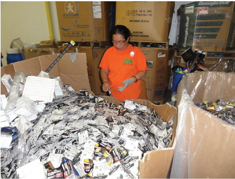
Figure 1. Battery separation: employee wears a cut-resistant glove to protect from knife cuts while removing batteries from the packaging. Photo by NIOSH.
