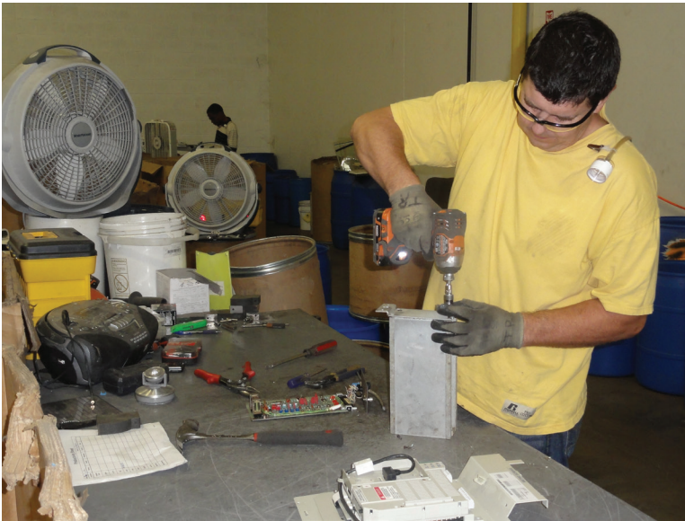
Figure 2. Employee using a cordless screwdriver in the demanufacturing process. Photo by NIOSH.
