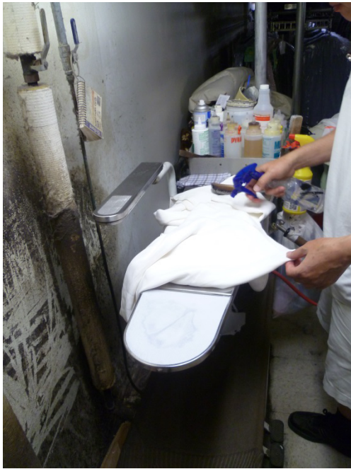
Figure 1. Employee spraying shirts with a SolvonK4 pretreating solution before drycleaning. Photo by NIOSH.
