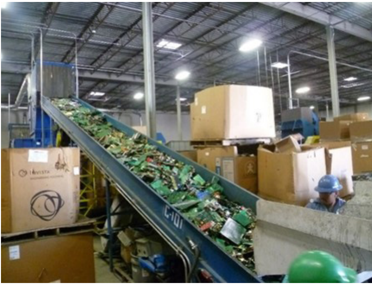
Figure 1. Electronic shredding conveyor. Photo by NIOSH.
