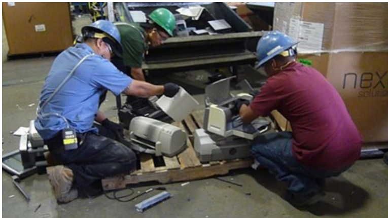
Figure 3. Three of the five disassembly employees manually disassembling printers. Photo by NIOSH.
