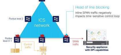
While this approach reduces the number of appliances required to provide full visibility, it still increases the amount of traffic going through the industrial network. Traffic is multiplied because you're duplicating traffic to SPAN it to a remote switch. And the more traffic on the network, the slower it becomes, resulting in jitter – often an unacceptable compromise in industrial networks where processes need to run faster and machines must be timely synchronized.
