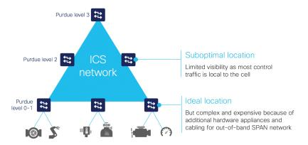
Some technology providers attempt to address this problem by leveraging remote SPAN (RSPAN). RSPAN allows you to duplicate traffic from a switch that doesn't have a sensor appliance to a switch that has one.
