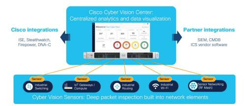
The benefits of Cisco Cyber Vision aren't limited to organizations with Cisco networks. The sensor can also be offered in a SPAN architecture with Cisco IC3000 hardware sensor appliance. This provides maximum deployment flexibility to meet your needs with your existing network, while giving you time to replace older switches with DPI-enabled network equipment that's capable of seeing everything that attaches to it.
