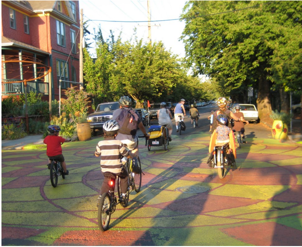
A Painted Intersection, planters, and curb extensions to reinforce that the street is intended for local, slow-speed use instead of cut-through vehicle traffic.
