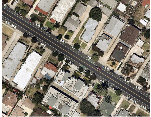
Before-and-after road reconfiguration on Duquesne Avenue. General Flow lanes were narrowed to make way for a Class II bike lane while retaining parking.
