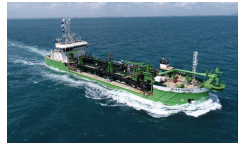
The compact trailing suction hopper dredger 'River Thames' ensures high manoeuvrability.
