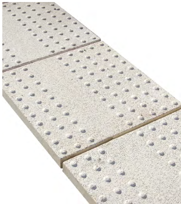
Tactile paver: two options; A) Sierra White Granite in 12" x 12" size; B) Hanover Tudor tactile paver in White, 24" x 24" size; pavers to be resolved with module of granite ramp pavers at full or half paver joints; evaluate both options at pilot block; make choice at final design.
