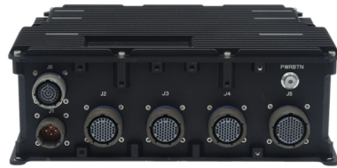
GEODE rugged computer system Internal construction features cable-eliminating I/O board (left) and conduction cooled COM-based CPU (right)
