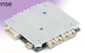
Rugged Ethernet switch used in robot
