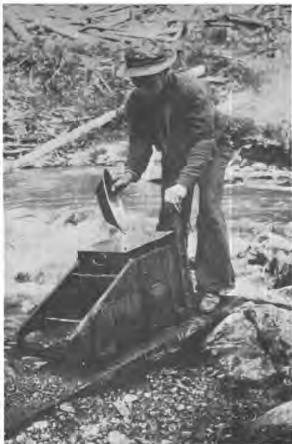
From 1855 to the early 1900's the rocker was often used in one- or two-man operations along gold-bearing bars of the Columbia River to separate placer gold from sand and gravel.
