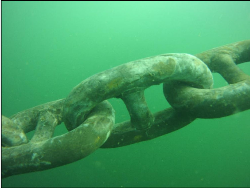
Photograph 11 : Underwater View of the Typical Clean Anchor Chain.
