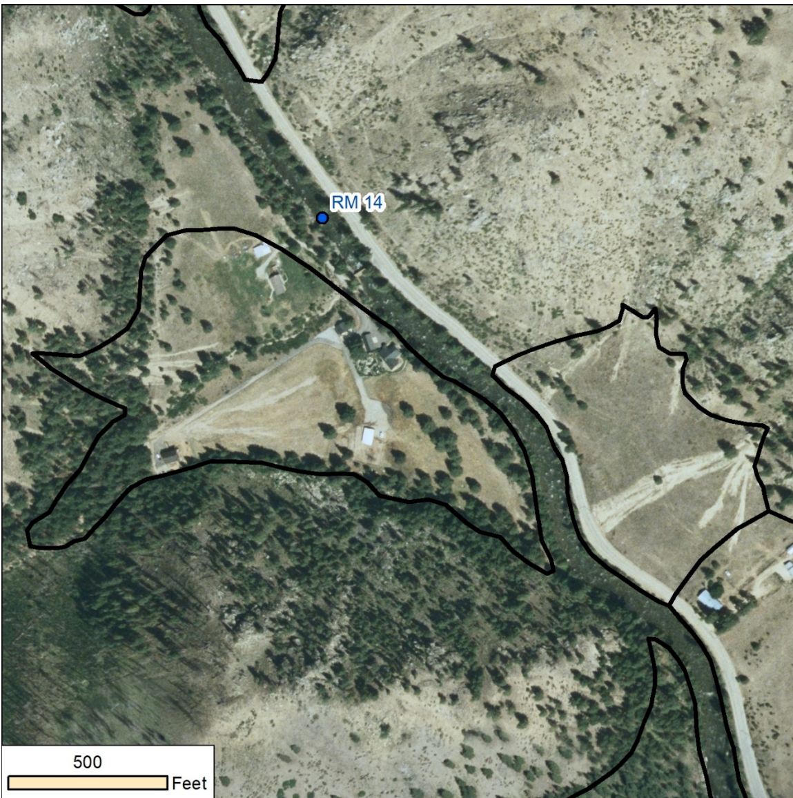
Figure 6. 2006 USDA photo of Tye Ridge Spring No. 1 fan and unnamed fan to the east showing impact from sediment onto the fans, from the 2006 event. This is obvious from light colored lobes on the fans.
