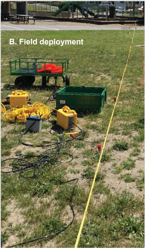
Figure A1. Processing and data acquisition flow for the active-sourced MASW method. A. Simplified schematic of an MASW geophone array. B. Photo of part of 48-channel geophone array deployment. C. Shot-gather of a shot in which the source is outside the array. The Rayleigh surface wave propagation is highlighted in red. D. Phase-velocity vs. frequency dispersion image with the trend of the fundamental mode of surface waves identified by black circles. The fundamental mode is identified as the high spectral amplitude (warmer colors) with the lowest phase velocity. For this dispersion image, the fundamental mode can still be identified despite higher modes. E. The final inverted 1D SVDP showing the measured dispersion curve (blue squares) and the modeled dispersion curve (black diamonds).
