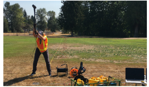
A WGS scientist generates seismic waves by striking a metal plate with a sledge hammer. The waves are recorded by an array of geophones visible on the ground in the background.
