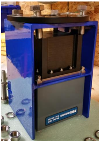
Figure 7. Close-up of R2Sonic 2020 multibeam sonar head (bottom, grey) and Applanix IMU (top, black) with mount (blue).
