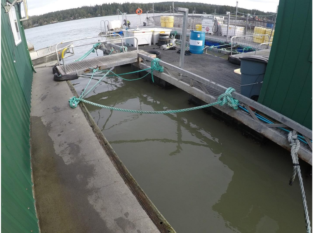
Figure C-86: South Side of Main Barge, Showing rafting of Intermediate Barge.
