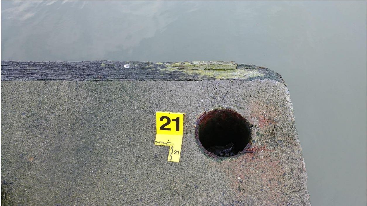
Figure C-60: Anchor #21, NE Corner of the Main Barge. Part of an Anchor Bridle System.
