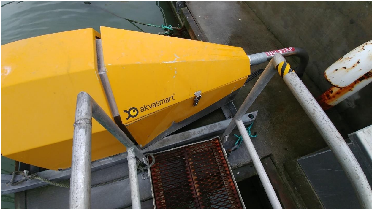
Figure C-88: Feed Blower Blocks Gangway between Main Barge and Feed Barge
