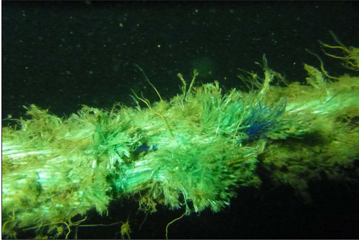
Photograph 31: View of Broken Strands in the Rope at Site 1 Anchor Line 7, Looking West.
