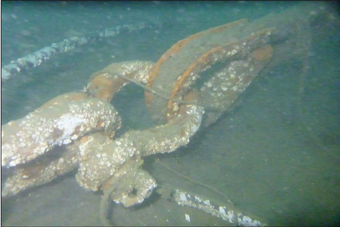
Photograph 15: View of the Rope to Anchor Chain Connection (Sleeve, Shackle and Thimble) and Random Piping at Site 1 Anchor Line 1, Looking North.
