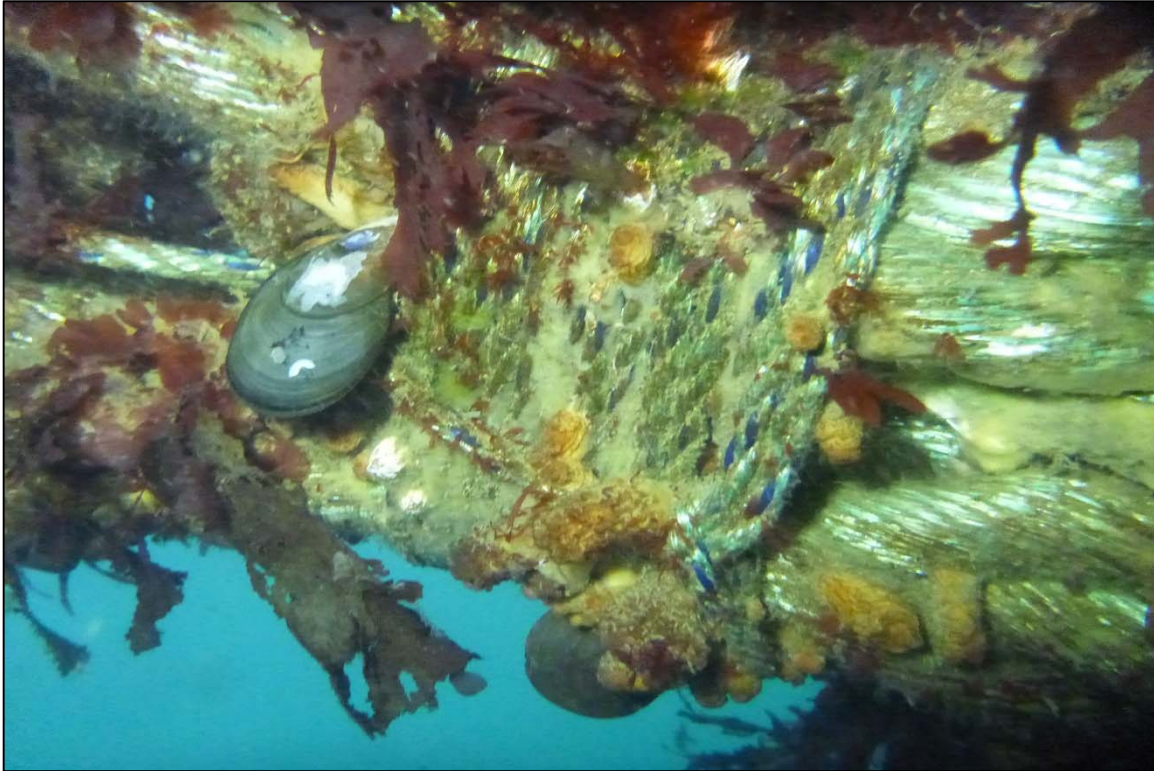
Photograph 79: View of the Lashings at the Upper Anchor Chain to Rope Connection at Site 1 Anchor Line 23, Looking South.
