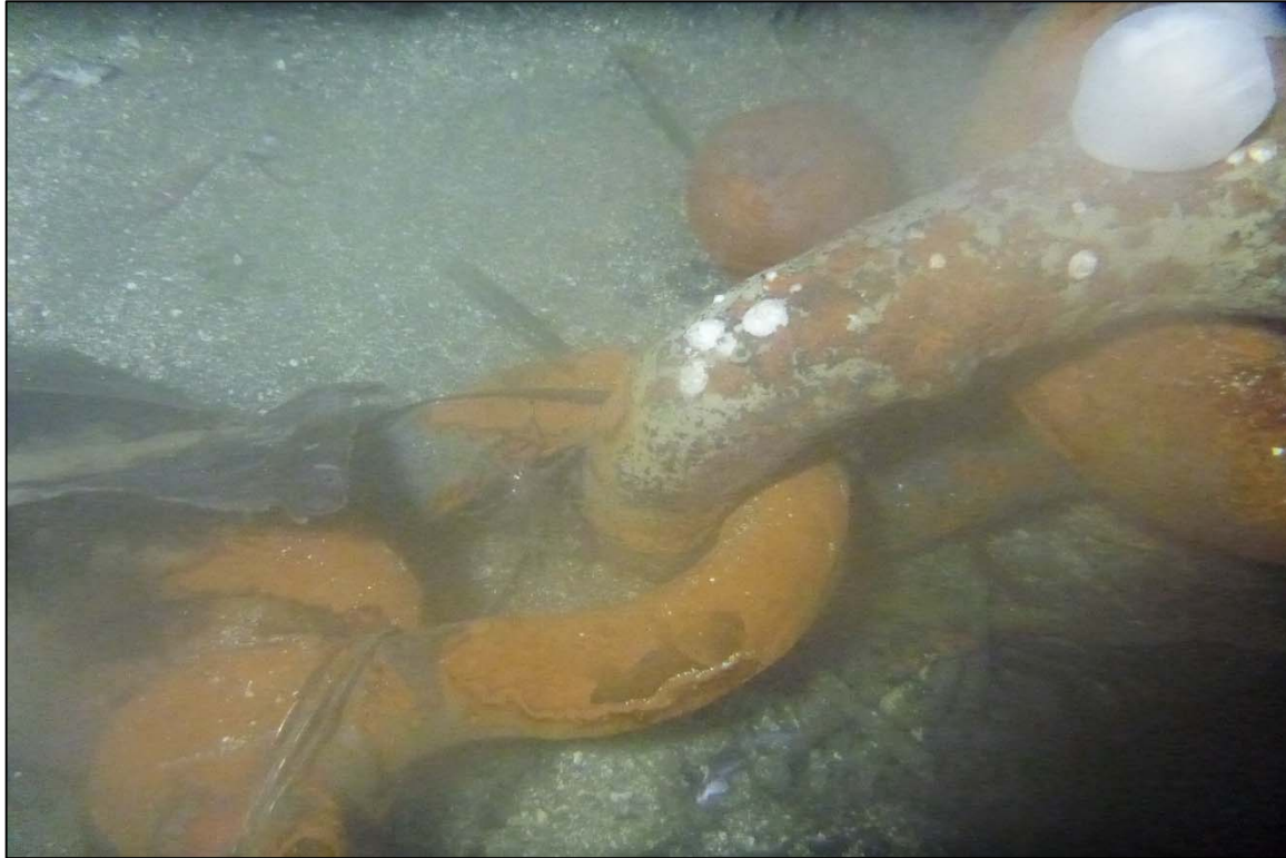
Photograph 11: View of the Lower Anchor Chain to Anchor Connection (Shackle) at Site 1 Feed Barge North Anchor Line, Looking West.
