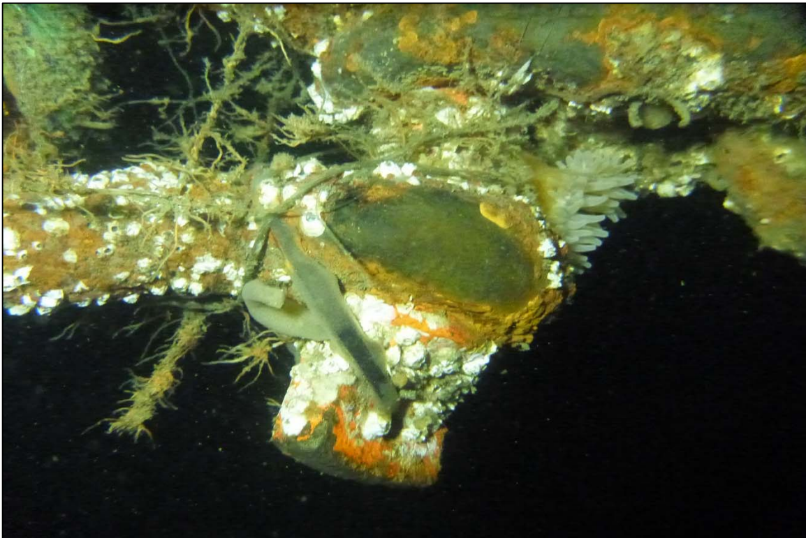
Photograph 46: View of Lower Anchor Chain to Anchor Rope Connection with Safety Zip-Tie at Site 3 Anchor Line 10, Looking Northeast.
