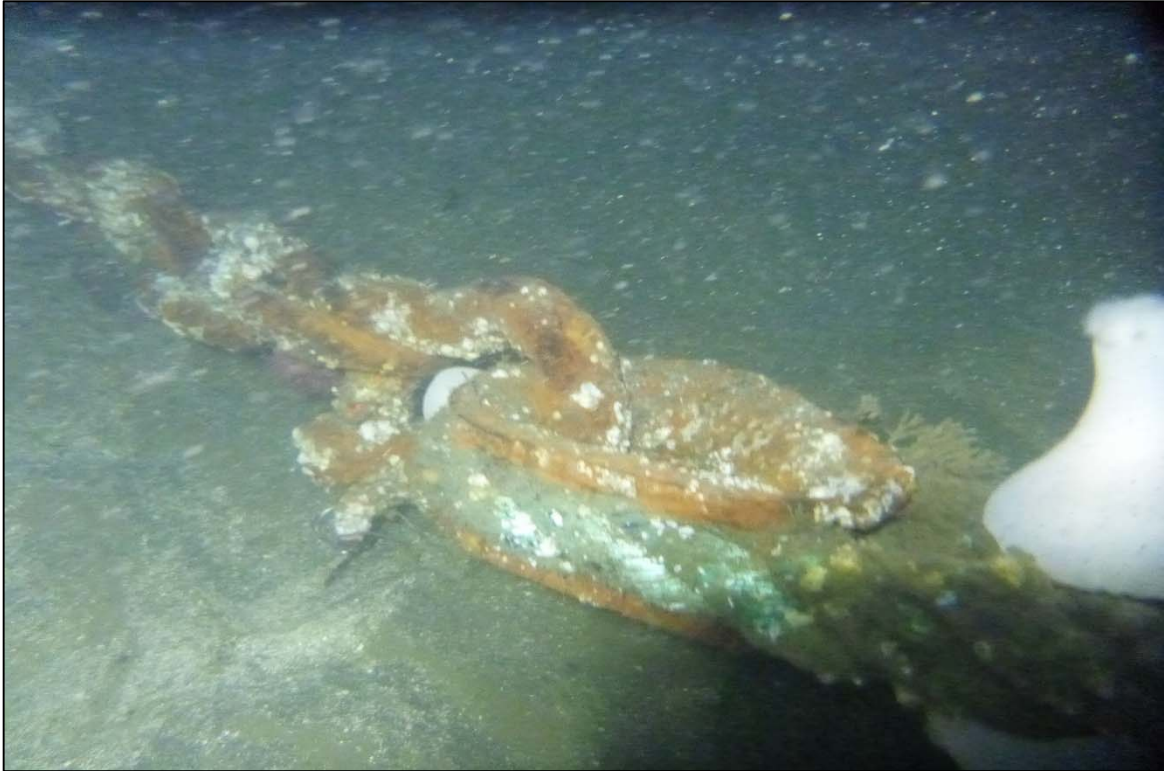
Photograph 49: View of Lower Anchor Chain to Anchor Rope (Shackle and Thimble) at Site 3 Anchor Line 11, Looking Northeast.
