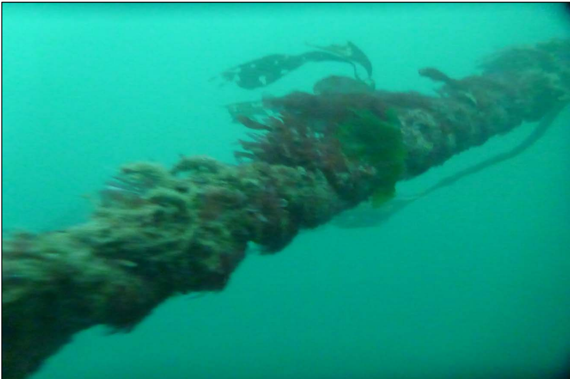
Photograph 48: View of Anchor Rope Heavy Marine Growth at Site 3 Anchor Line 11, Looking North.
