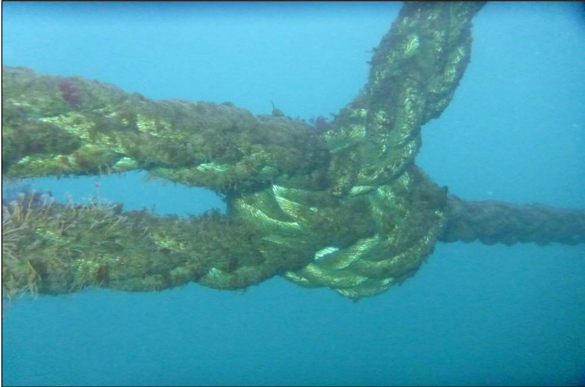
Photograph 51: View of Upper Anchor Rope Condition (Bowline Knot) at Site 3 Anchor Line 12, Looking Northeast.
