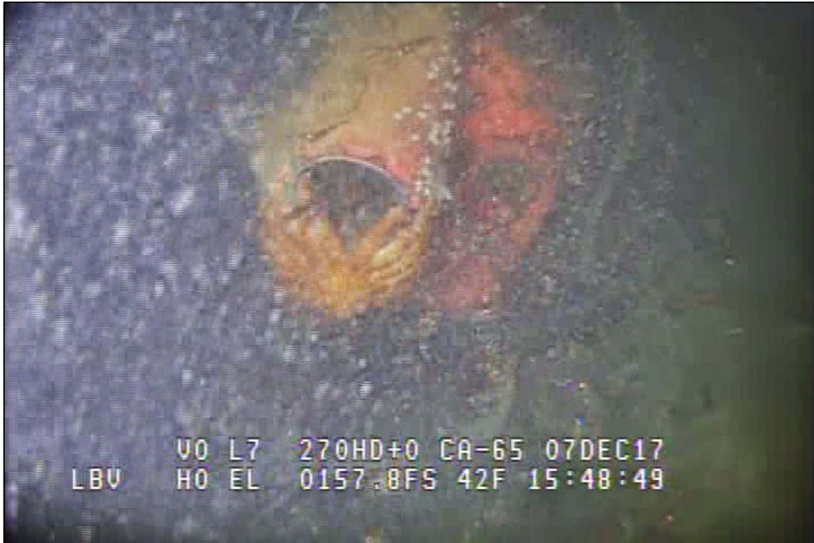
Photograph 60: View of Buoy and Ropes in the Channel Bottom where Lower Anchor Chain is Embedded at Primary System Anchor Line 16, Looking West.
