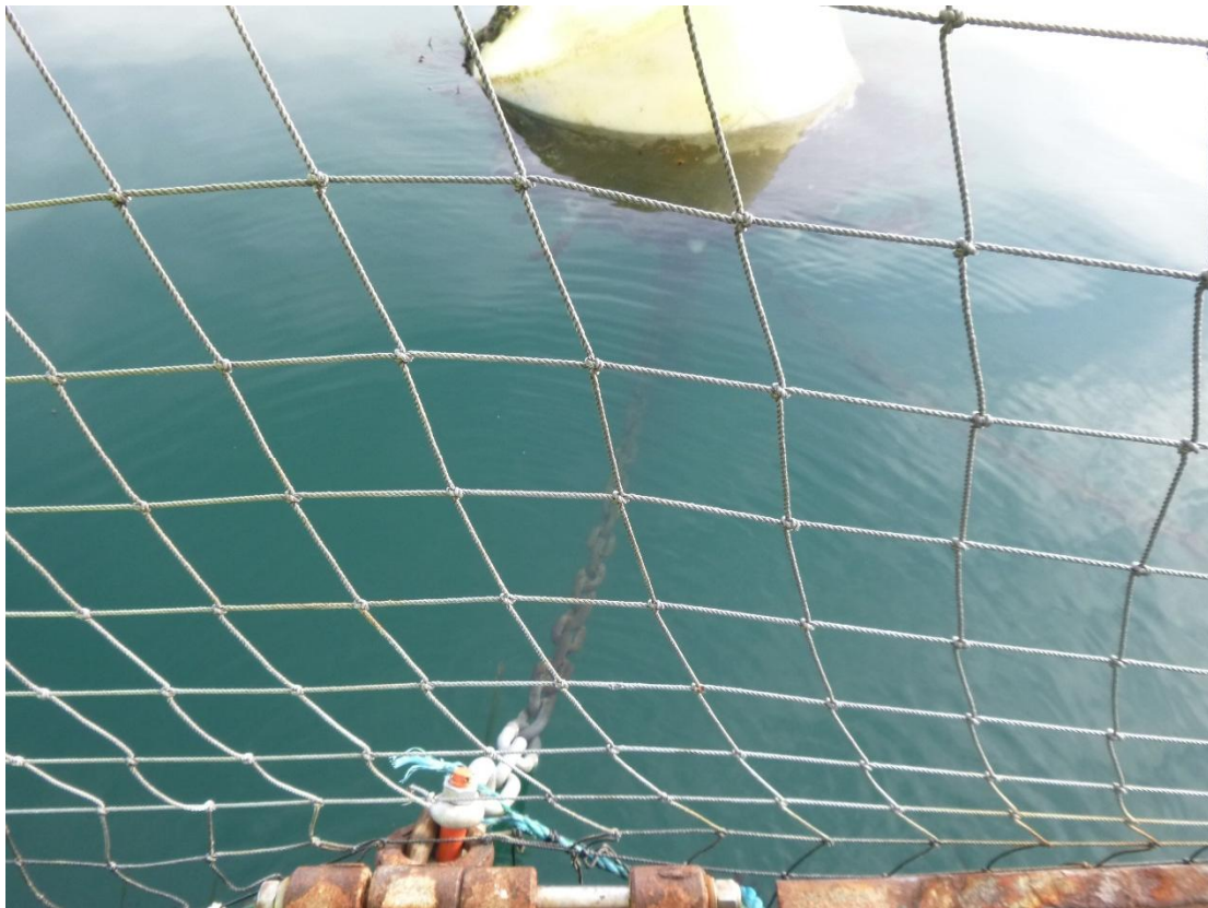
Figure C-12: Anchor 4 Bridle Chain and Buoy
