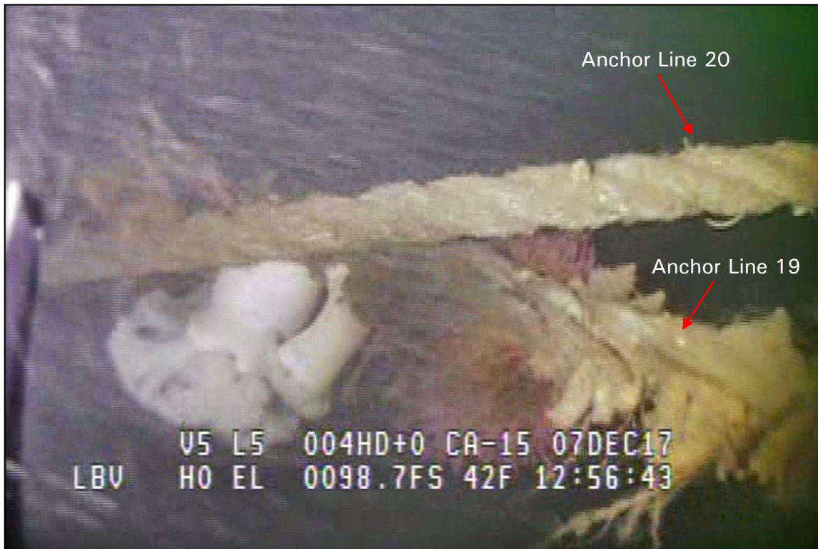
Photograph 62: View of Anchor Line 19 Crossing Below Anchor Line 20, Looking North.
