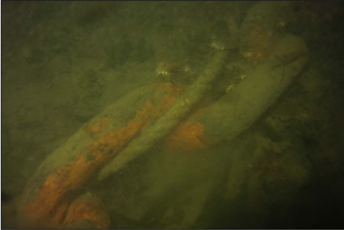
Photograph 35: View of the Anchor Chain on the Channel Bottom at Anchor Line 21 (Typical Observed by Diver), Looking North.
