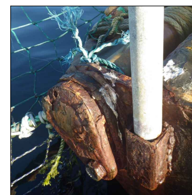
PHOTO 9 SEIZED HINGE AT ANCHOR 13
