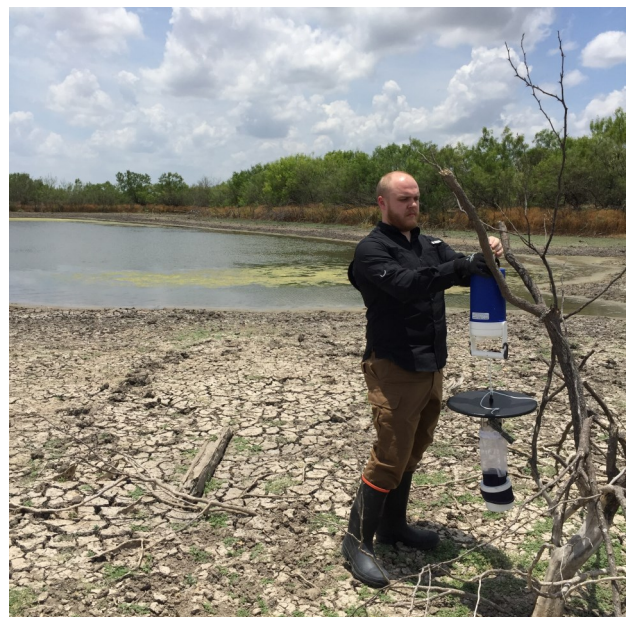
Figure 2: Trevor Maness Setting up a CDC Light Trap
