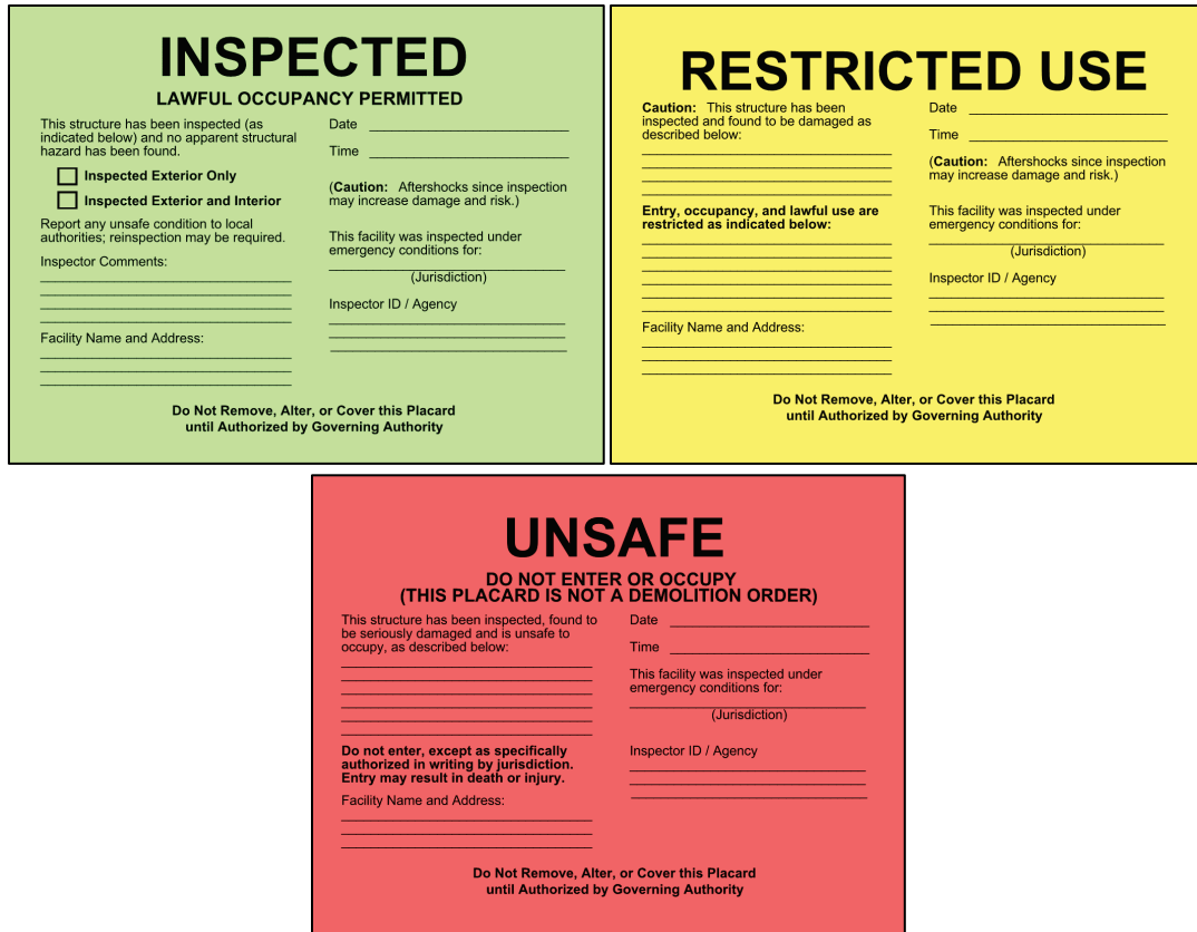
Figure 2-1 INSPECTED, RESTRICTED USE, and UNSAFE placards from ATC-20-1.
