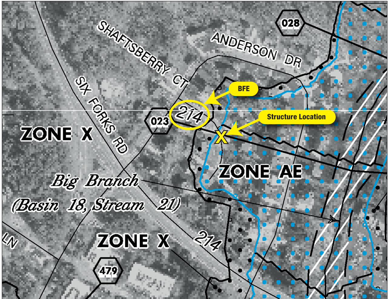
Figure 2-3. Building and stream location on a FIRM
