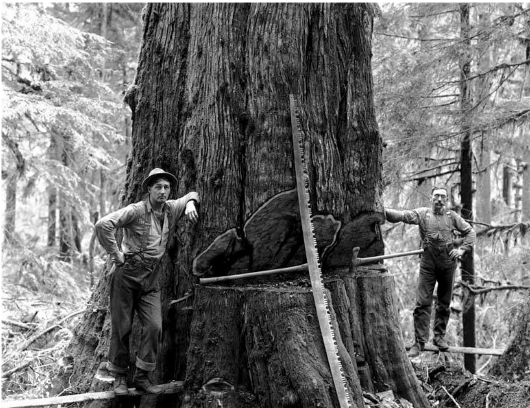
Figure 3-4 Tree notched to define direction of fall (image from public domain).
