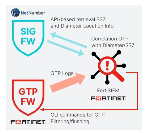
The FortiSIEM correlates the GTP source with the last known device location and can instruct the FortiGate GTP Firewall to reject the GTP session in case a violation is detected between the GTP source and the last known end-user location.
