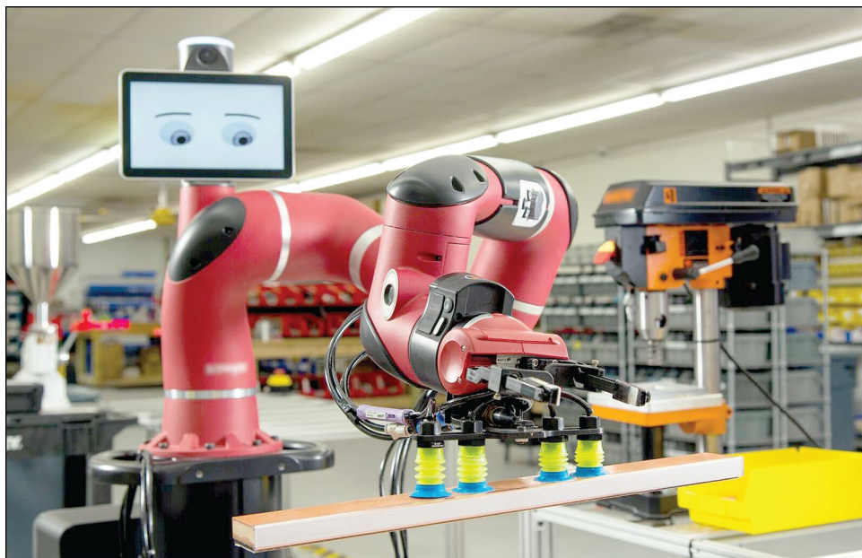
Figure 6: Collaborative Robot Lifting Piece of Wood Prior to Cutting
