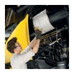
Convenient access to engine air filter.
