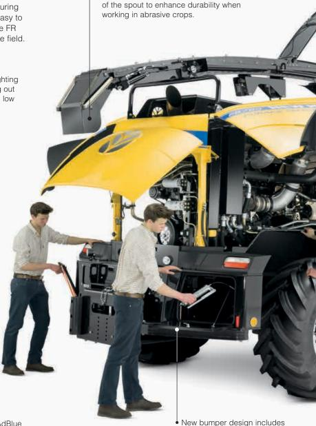
Heavy-duty wear-resistant plates can be fitted in the crop flow and on the full length
