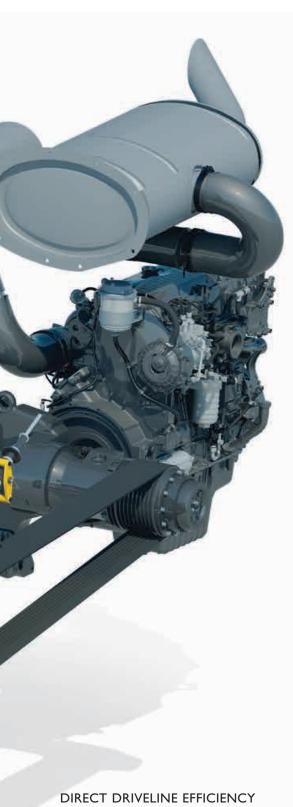
The single drive belt transmits 100% of the available power to the cutterhead, crop processor, and blower for ultimate forage chopping efficiency. The FR780 and FR850 are fitted with heavy-duty 9HB V-belt drives to transfer every last drop of performance. The main drive clutch is easily serviced, if needed, right from ground level.
