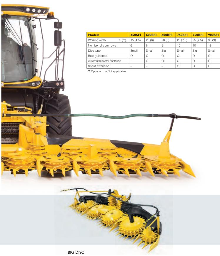
For harvesting tall, high-yielding corn, the large disc corn header is the best choice. Available in eight- or ten-row versions, the 53"-diameter discs cut through the tallest crops. These headers also work very well in wide-spaced corn and heavy-stemmed biomass crops.
