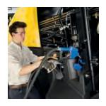
The fuel and 52-gallon AdBlue tanks are conveniently located next to each other to facilitate simultaneous filling
