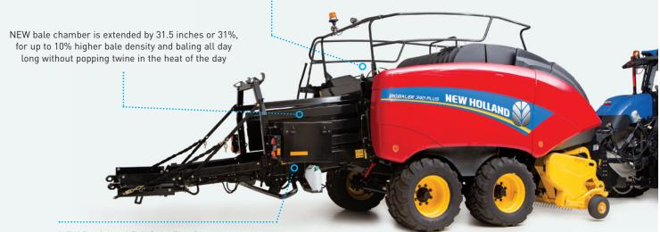
NEW Partial and Full Bale-Eject™ systems feature an active teeth system for more durability and reliable bale ejection
