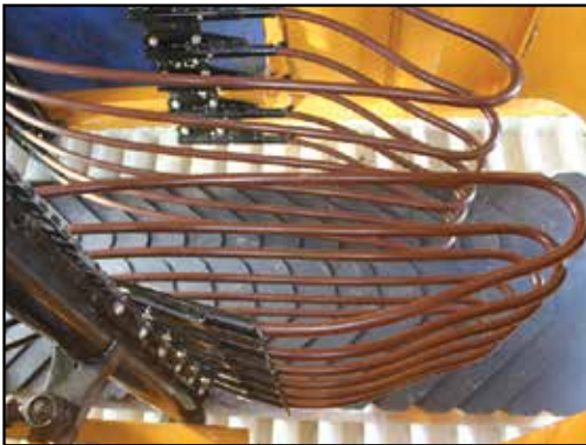
Oxbo Soft-touch bow rod head with extended contact rods
