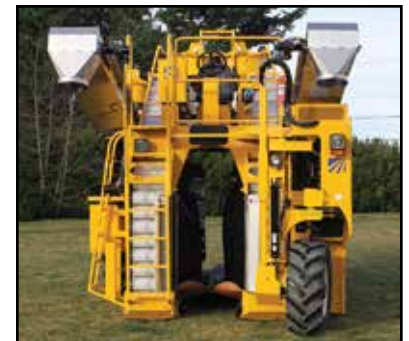
Oxbo double OTRC design for continuous tray raisin harvesting
