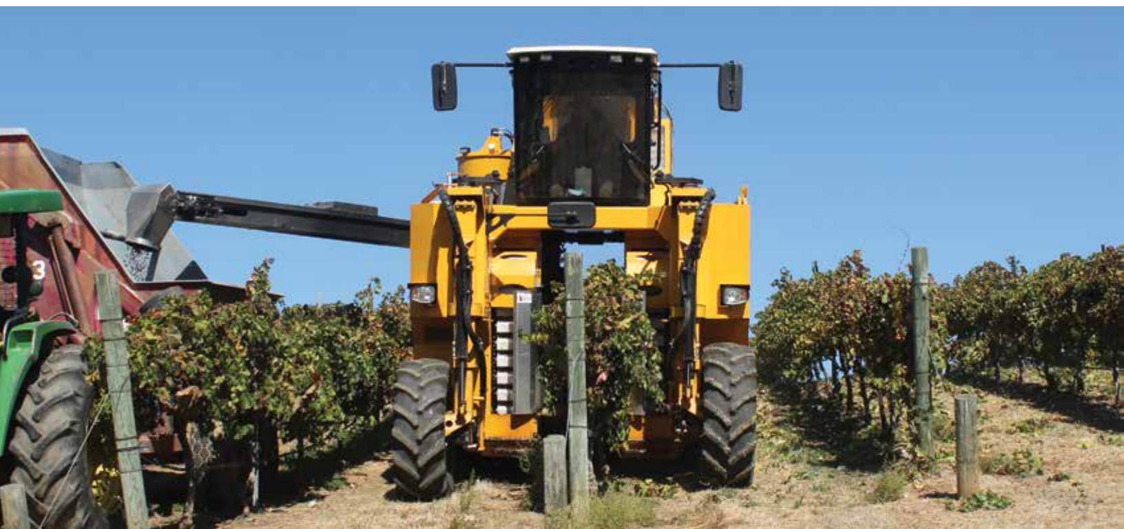
Oxbo double OTRC design for continuous tray raisin harvesting
