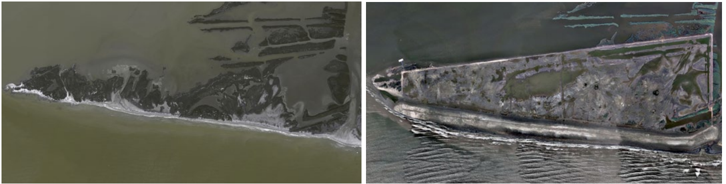
Overhead aerial photos of marsh creation behind a restored barrier island in Barataria Bay, Louisiana ( DIVER ID 35 ) in 2016, prior to construction (left image) and in 2018, 1 year after completion (right image).
