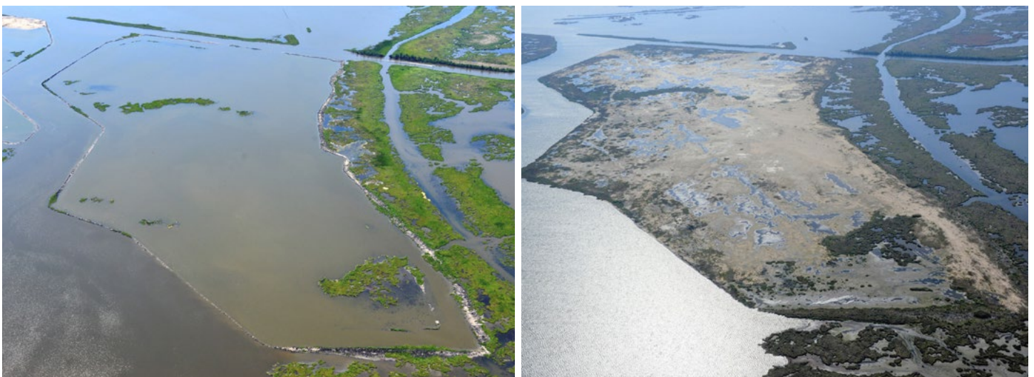
Louisiana Lake Hermitage Marsh Creation ( DIVER ID 4 ) before dredge placement in 2013 (left) and post-construction in 2015 (right).
