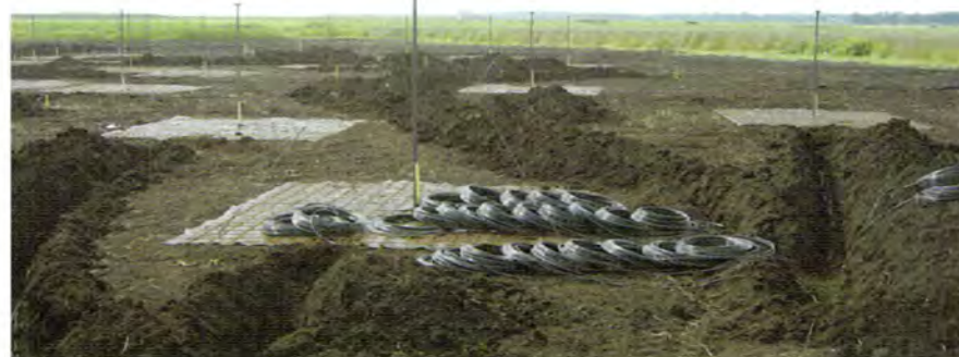
The first 13 of eventually 7,392 dipole antennas that will make up the LOFAR radio telescope. The area immediately around the antennas will revert to a nature reserve.
