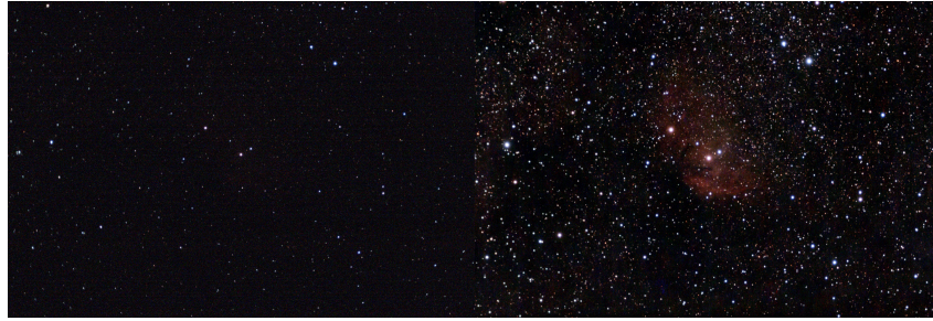
Figure 1: Observation of the Sh2_101 nebula with a Stellina automated telescope (night of 31/7/2022) [4]. The image on the left corresponds to a single 10s exposure frame and the image on the right is the result of the stacking of 340 frames (10 s exposure too).
