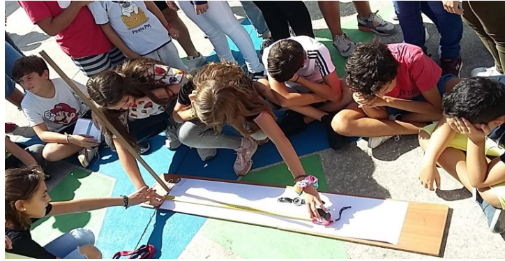
Figure 1: Measurement of the shadow of a vertical pole at solar noon to determine Earth's perimeter (Eratosthenes' experiment).
