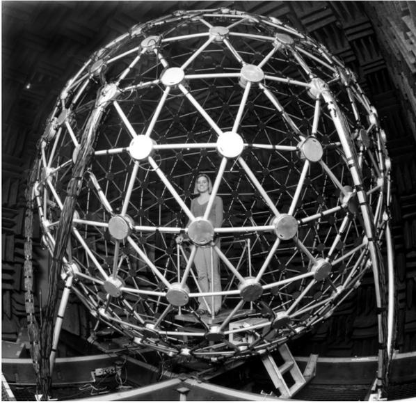
Figure 1: Auditory Localization Facility (ALF) where the experiment was conducted
