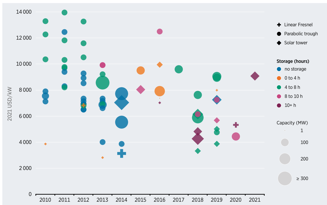
Figure 5.3 CSP total installed costs by project size, collector type and amount of storage, 2010-2021
