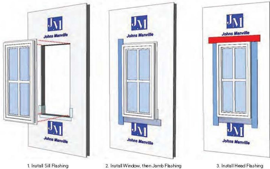
FIGURE 4. TYPICAL PENETRATION FLASHING DETAIL - FLANGED
