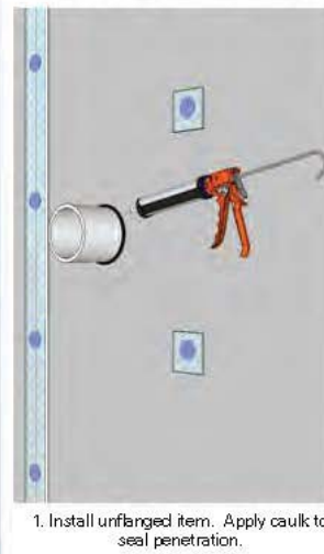
FIGURE 5. TYPICAL PENETRATION FLASHING DETAIL - UNFLANGED
