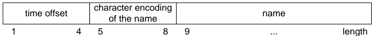
Figure 37: The data field of SLMetadataInfo Structure containing the value corresponding to a KhronosSeekPoint key.
