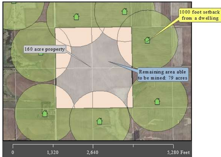
Figure 7. Conceptual map displaying a 160-acre parcel with 1,000-foot setbacks drawn around surrounding dwellings. Note the limited area between the circles.
