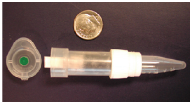
FIGURE 7. A centrifugal filter device consists of a 5 µm basket filter (left portion), and a detachable assay tube (right portion), shown here with a dirty sample swab inserted in the filter basket.
