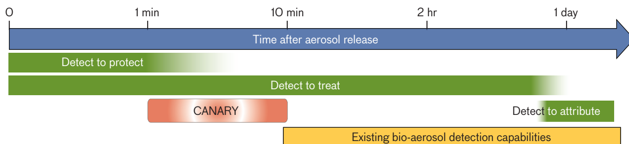
FIGURE 1. CANARY's (Cellular Analysis and Notification of Antigen Risks and Yields) rapid response uniquely enables coverage into the detect-to-protect region for an aerosol release.
