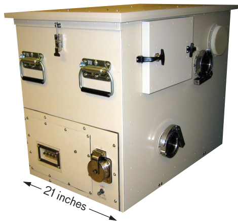
FIGURE 16. The transportable BCAN sensor, shown on left, produced the data for several cases typical of CANARY analysis of a particular threat (an indoor/outdoor study of Lincoln Laboratory, an outdoor test at Hill Air Force Base, and an indoor test in a District of Columbia office building). The resulting receiver operating characteristics (ROC) graph on the right shows the comparison between false-alarm rates and the probability of identification on the basis of a single test. In each curve, n is the number of tests at that specific test site. ACPLA stands for agent-containing particles per liter of air.
