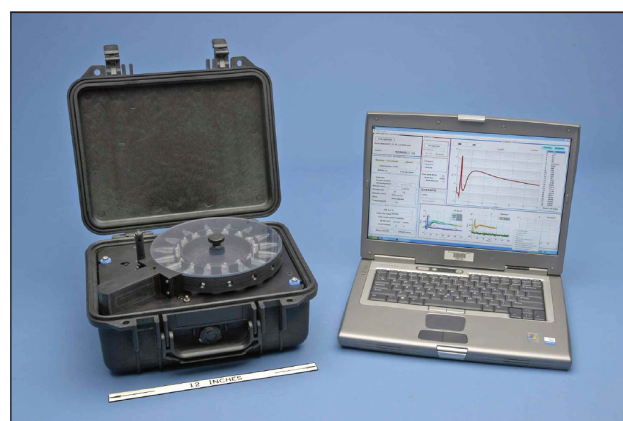
FIGURE 6. The portable 16 channel CANARY sensor is built into a light-tight and water-tight case and contains provision for conversion to battery-powered operation. The laptop is used to operate the sensor with custom software written to simplify collection and organization of sample and reagent information, as well as perform automated identification based on signal characteristics.
