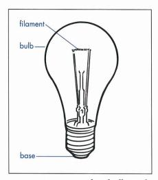
Incandescent lamps convert electric power into light by passing electricity through a filament of coiled tungsten wire, heating it until it glows. The lamps usually are filled with an inert gas mixture consisting primarily of argon. Of the energy that goes into the incandescent filament, only 10 to 15 percent is emitted as light; the rest is emitted as heat.
