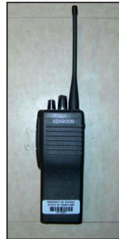
The only acceptable narrowband-capable portable radio is the Kenwood TK 390, pictured here.
