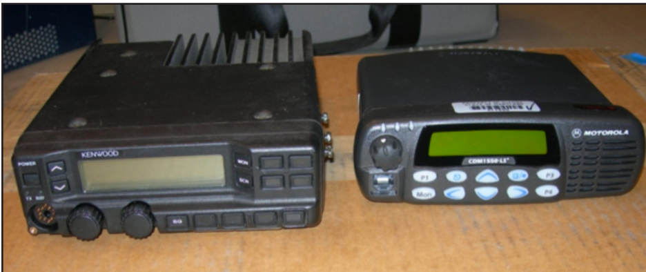
Acceptable narrowband-capable mobile radios are the Kenwood TK 890 (the KCH-11 model is shown) (left) and the Motorola Model CDM 1550 (right).
