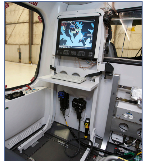
The tactical flight station in the AW-139 provides a searchable database with the ability to identify any location or address and links to the Wescam MX-15i camera, TrakkaBeam 800A search light, and flight management system (autopilot) for aircraft navigation.
