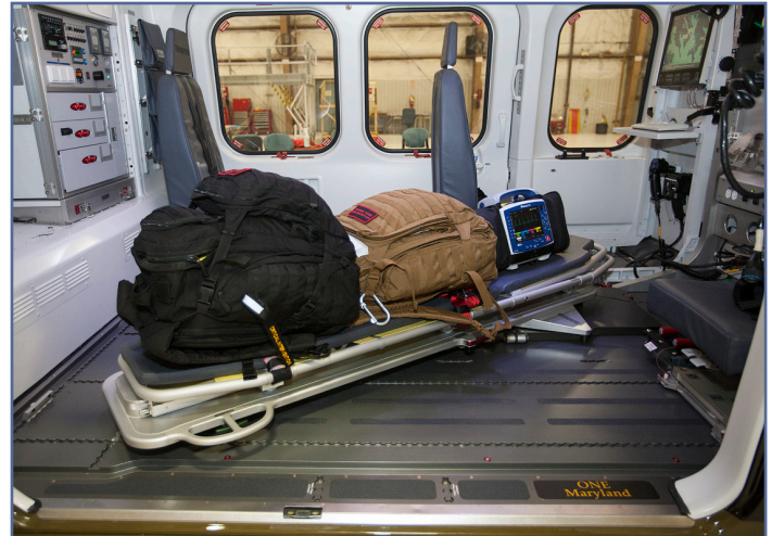
In the AW-139, all patient loading takes place from the RIGHT SIDE of the aircraft. The primary patient is loaded HEAD FIRST.
