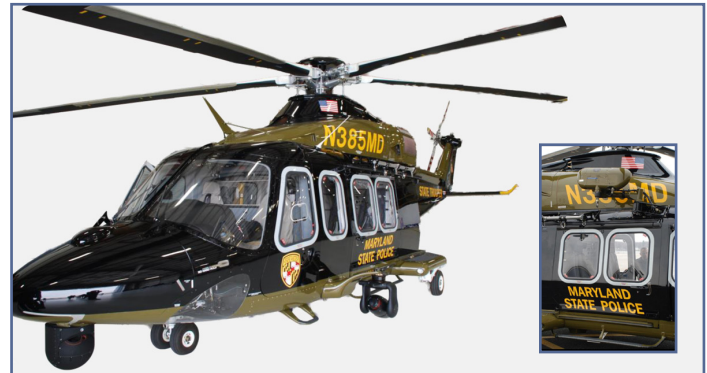
The Goodrich® Type 1 retractable hoist unit features 300 ft. of spin resistant cable, a 600 lb. lifting capacity, and operates at 250 ft. per minute.
