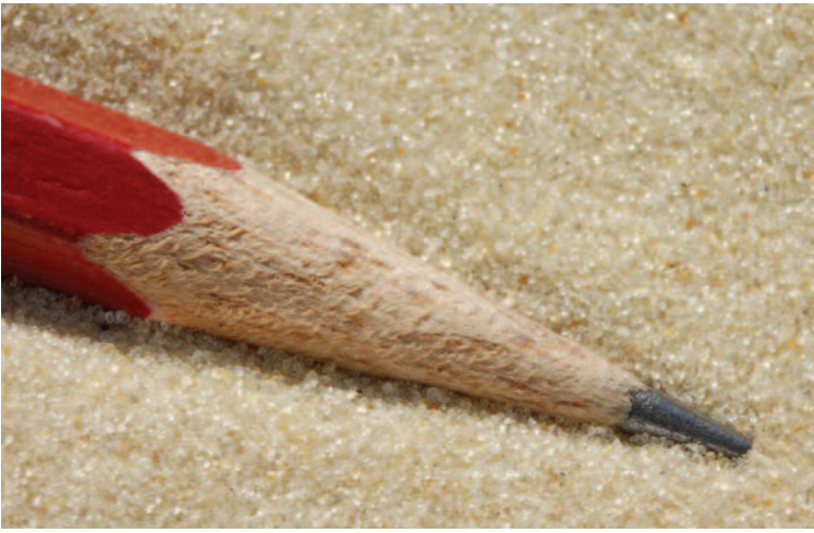
The best frac sand consists of tiny, rounded grains of nearly pure quartz.
