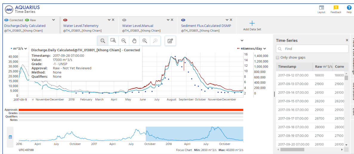
Figure 26: Visualization of time series data for QC using new tools such as AQUARIUS.
