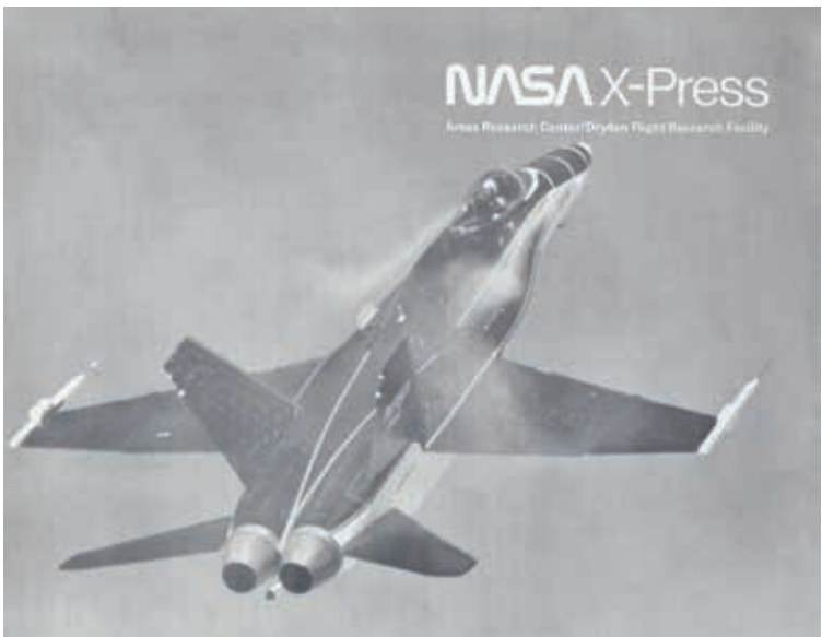
The Sept. 29, 1989, X-Press featured a cover of the F/A-18 High Alpha Research Vehicle conducting flow visualization studies with smoke. A second phase of HARV research included engine nozzles that could direct thrust for control in flight regimes that ordinary aircraft could not travel.
