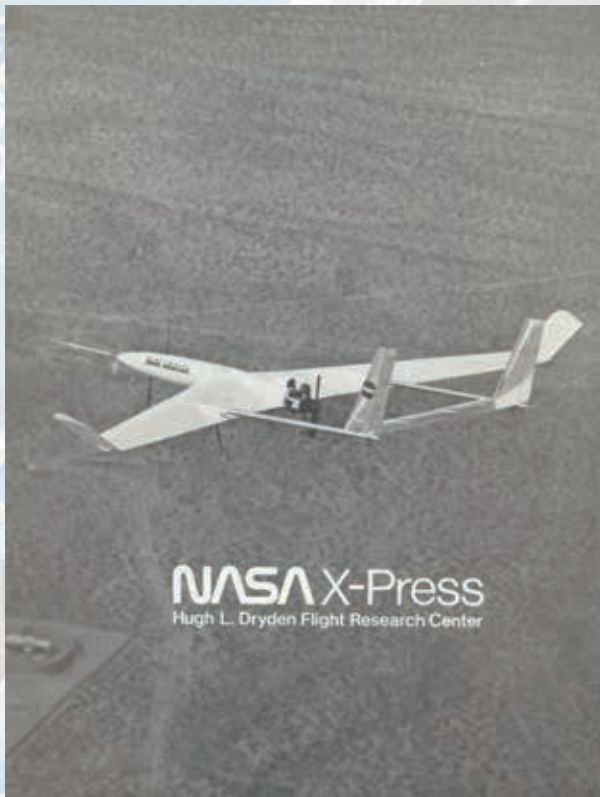
The propeller-driven Mini Sniffer was envisioned as a remotely piloted vehicle to collect atmospheric samples in the upper atmosphere. A later hydrazine-powered engine was intended to gather samples of rock and data from Mars after being dropped by a spacecraft. This was the cover of the Jan. 13, 1978, X-Press.
