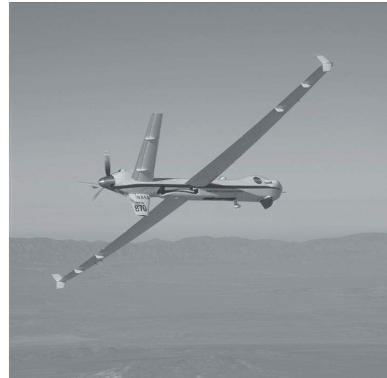
The Ikhana aircraft is flying a TAMDAR Edge probe that could significantly improve weather models and forecasts.
