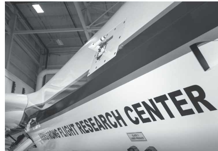
The Ikhana aircraft is flying a TAMDAR Edge probe that could significantly improve weather models and forecasts.
